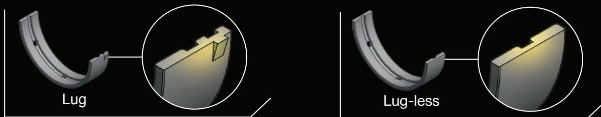
For aftermarket installers, placing a lug-less bearing into its correct position requires additional accuracy and attention to details. Shell and housing should be aligned for unimpeded oil hole orientation and for proper centering to avoid bearing-to-crank fillet ride.
