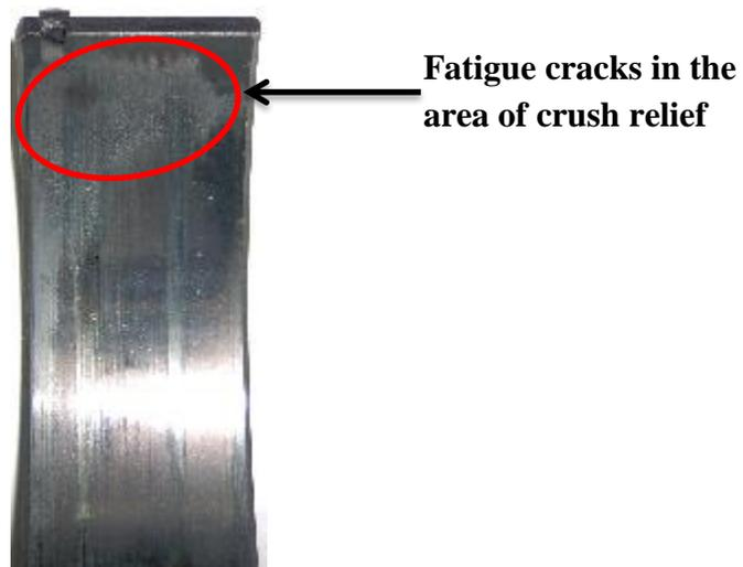
**Fig.7 Fatigue cracks in the crush relief area**
